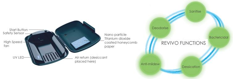
ACS Revivo is a portable electronic device designed to remove the harmful moisture and bacteria that can penetrate into any electronic device worn in the ears. The special high-speed fan circulates air inside the Revivo and capture moisture via the replaceable silica gel desiccant pack. Nano particle Titanium dioxide and UV photocatalytic reactions generate hydroxyl radicals and negative oxygen ions to both sterilize and sanitize the devices.
